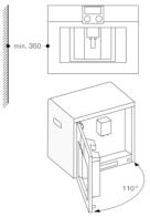
If using the 92° door hinge restrictor (spare part no. 00636455), the minimum distance from the wall is only 100 mm.
